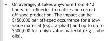
• In-line viscometers allow immediate adjustments whenever the viscosity goes outside the control band, improving the quality of the distilled lubricant. Maintaining tighter control on viscosity can result in a 0.5% production improvement, or \$50,000 in profit per line each month.
